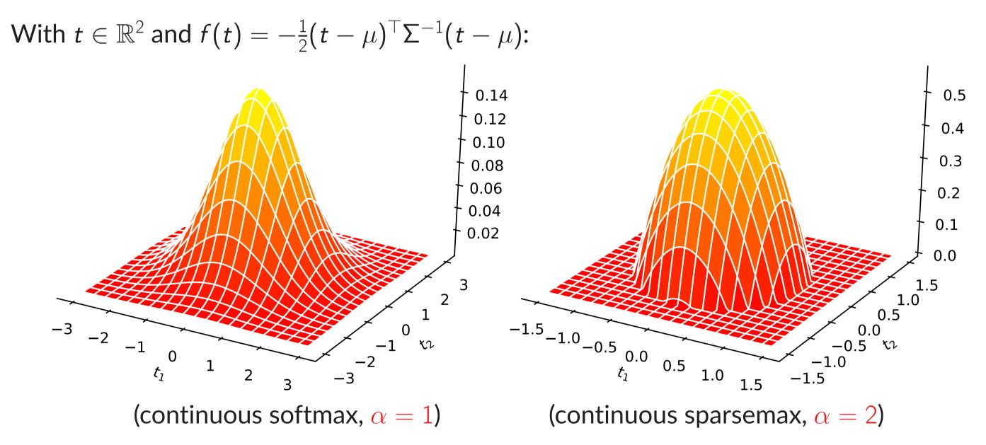
Truncated paraboloid has sparse, varying support!
